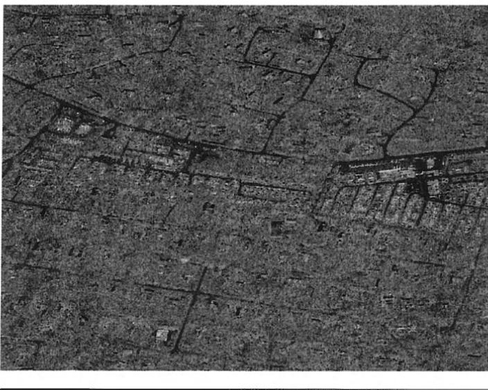
Fig. 3. Cloude-Pottier mean alpha angle,  $\bar{\alpha}$  in degrees. In accordance with remarks in Section I and with Fig. 2, roads have low values for  $\bar{\alpha}$ , vegetation has  $\bar{\alpha}$  around  $45^\circ$ , and parts of most of the buildings and caravans have very low or very high values (single or double bounce).
